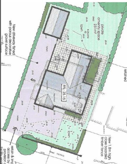
with a single storey detached garage abutting the boundary with the application site. The neighbouring dwelling has no windows on the gable. A new 1.8m high close boarded timber fence will be provided along this particular party boundary from the garage to the road edge. The existing boundary planting will be retained to the rear of the dwelling.
