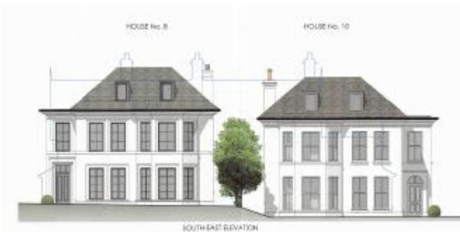
The dwellings will have a ridge height of 10.6m high above ground level with a hipped roof. The units will be finished in white sand cement render with hardwood sliding sash windows and a natural slate roof. The dwellings have a vernacular emphasis on the windows and an
