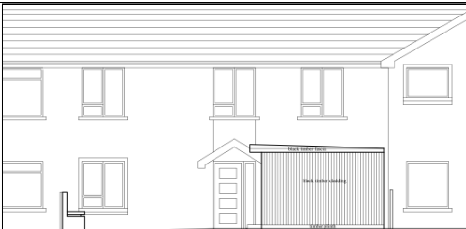
Front elevation showing shed to front of house
