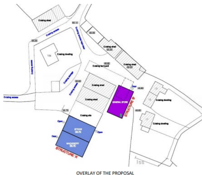
Figure 4 Proposed site plan showing the proposed buildings Structure A (coloured blue) and Structure B (coloured purple).
