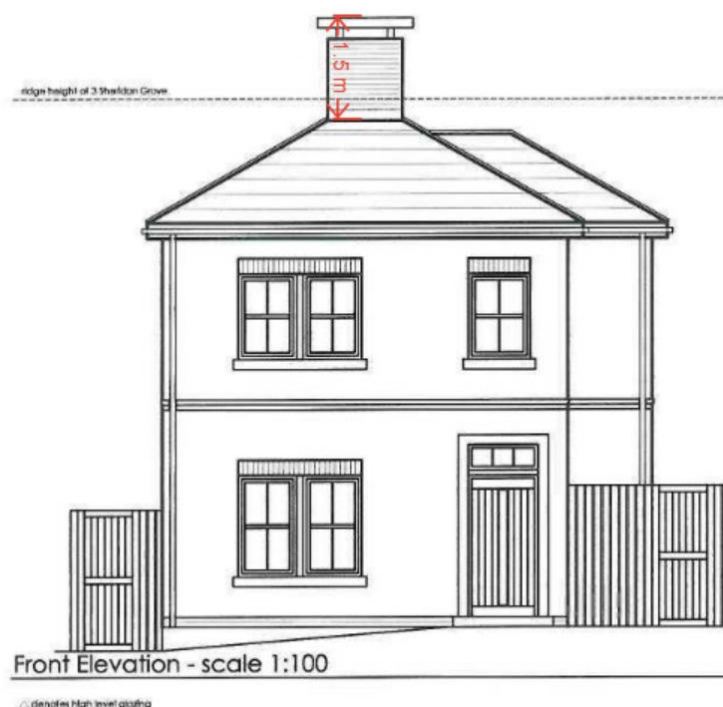
Figure 4 – Height of chimney on original design
