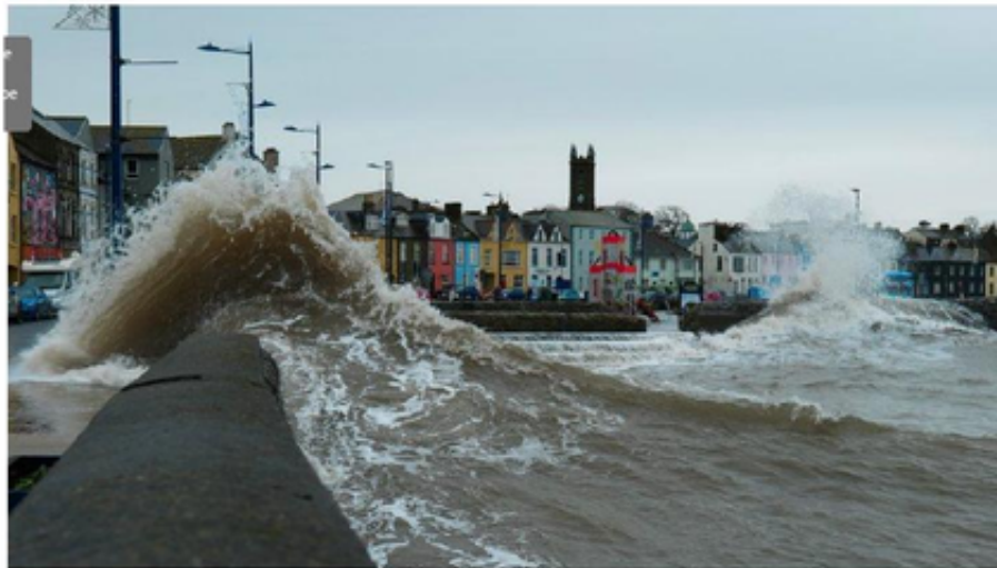
Example of oblique waves becoming “focused” and running along the existing sea defence at the inner parade, east of lemons wharf.
