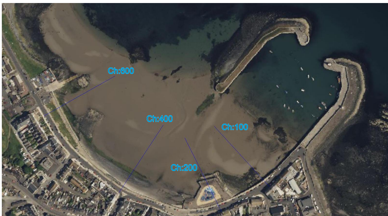
Figure 6-6: Locations of representative sections for overtopping
